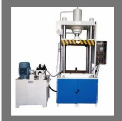
500 x 500 mm Compression Moulding Machine, 200 Tons
