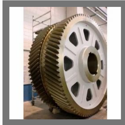
Heavy Duty Gear 3Meter/ 30 Module
