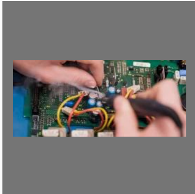
Vfd Drive Repair
