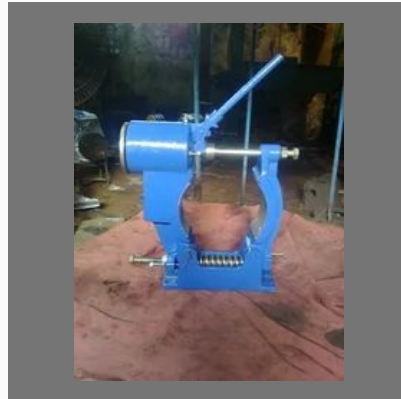
Elevator Brake Unit
