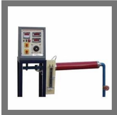
Heat Transfer Through Composite Wall
