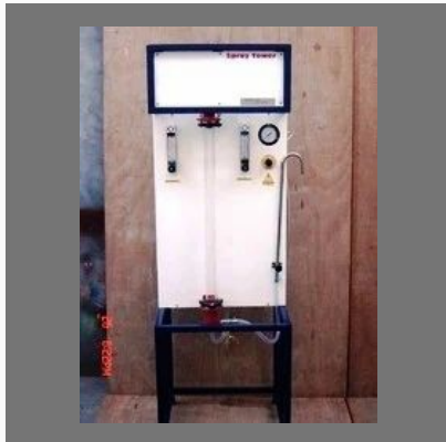
Spray Tower Apparatus
