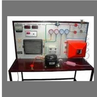
Air Conditioner Test Rig
