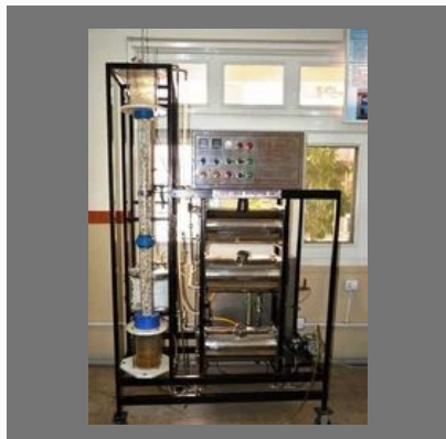
Liquid-Liquid Extraction in Packed Tower
