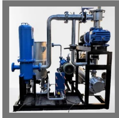
Mechanical Vacuum Booster System
