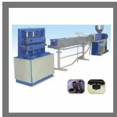
PVC Plumbing Pipe Plant
