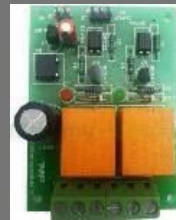
Two Relay Driver 5 v
