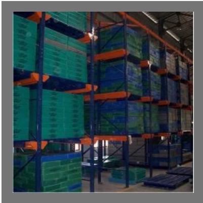
Storage Drive In Racking System
