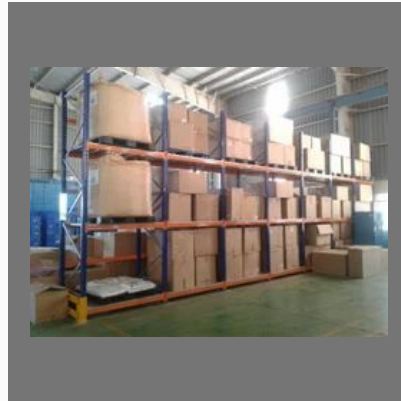
Conventional Pallet Rack
