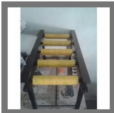
Gravity Roller Conveyor
