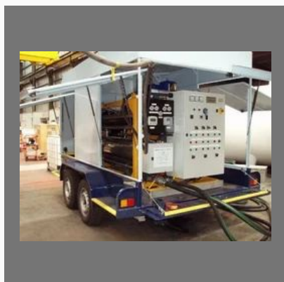
Transformer Oil Filter Machine Repairing Service
