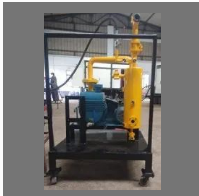
TRANSFORMER EVACUATION SYSTEM
