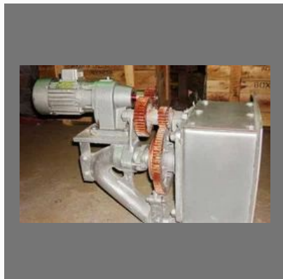
Manually Operated Rotary Soot Blower
