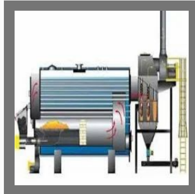
Waste Heat Recovery Boilers
