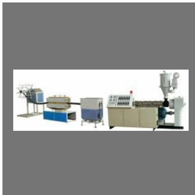
HDPE And PP Pipe Extrusion Plant
