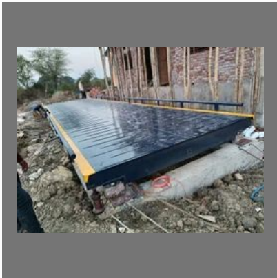
Top Loading Pit Less Weighbridge
