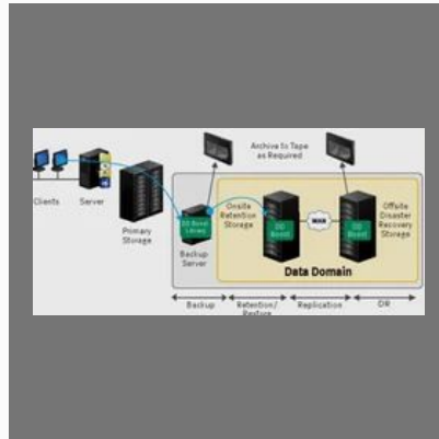
EMC Data Domain Server Backup
