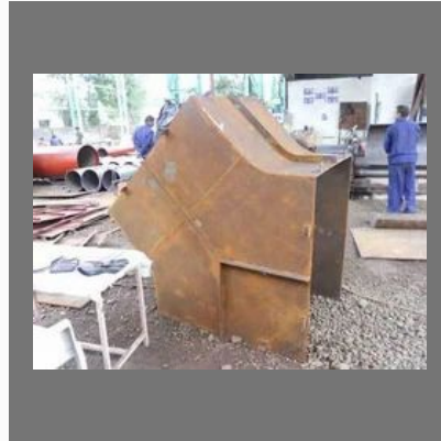
Mild Steel Ducting
