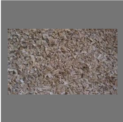
Grinded PVC Pipe Scrap
