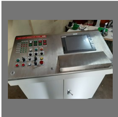
Plc Electrical Control Panel
