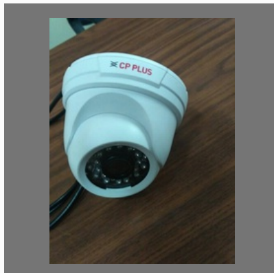
CCTV Dome Camera
