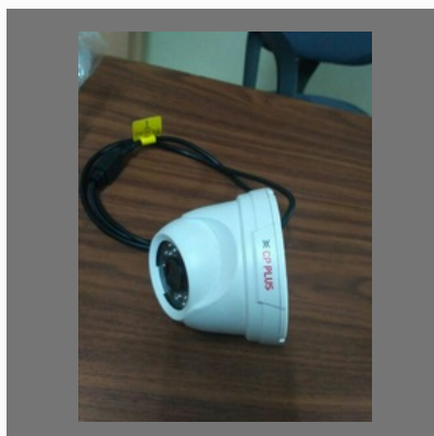
CCTV Dome Camera
