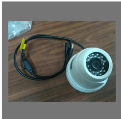
CCTV Dome Camera
