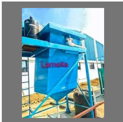
Lamella Clarifier System
