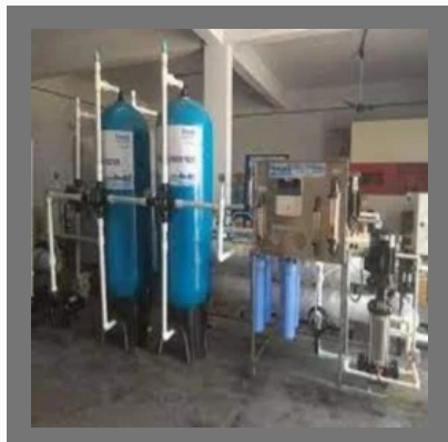
Reverse Osmosis Systems
