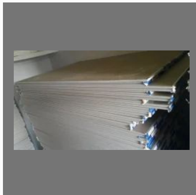
False Ceiling Gypsum Board
