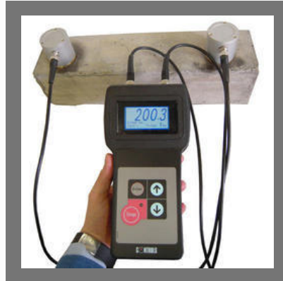
Ultrasonic Pulse Velocity Testing Service
