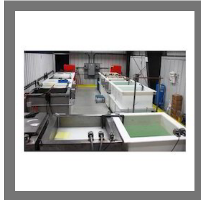
Tin Electroplating Plant
