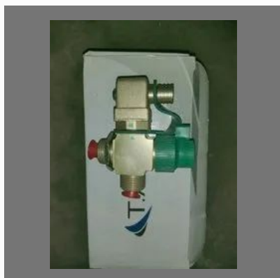
CNG Refilling Valve
