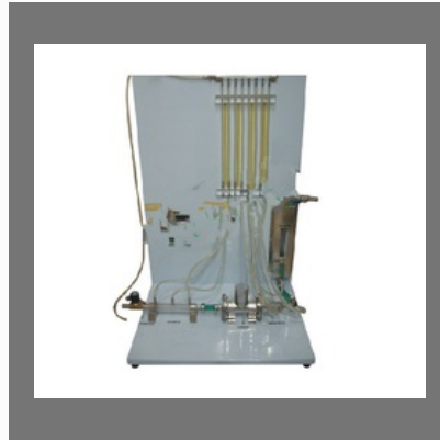
Computerized Flow Meter Calibration Equipment
