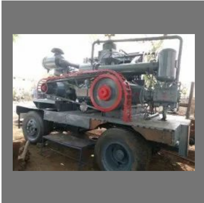
Borewell Diesel Engine Compressor
