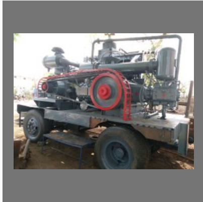
Borewell Diesel Engine Compressor
