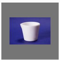
Evaporating Dishes Conical Shape With Spout
