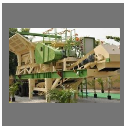
Mobile Crushing and Screening Plant
