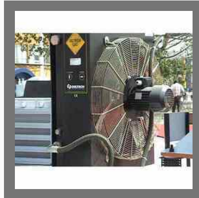
Air Oil Cooler
