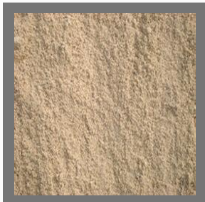
Boiler Bed Material
