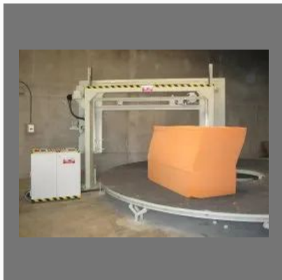
Box Foaming Plant
