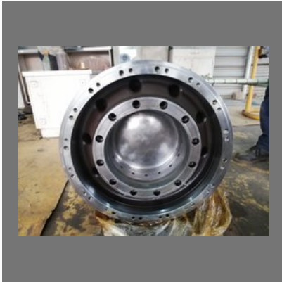
Mitsui Man B&w S60mc Piston Crown
