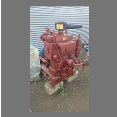
Tanabe Main Air Compressor H-73 , H-74 , H-273, H-274, H-373
