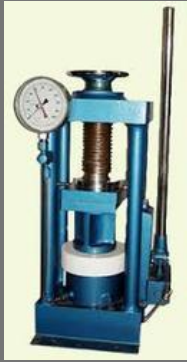
Cube Testing Machine 100 Ton Capacity Hand Operated
