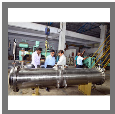
Heat Exchanger Condenser
