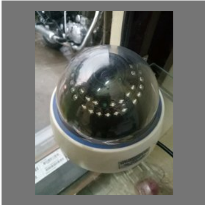
Office CCTV Camera
