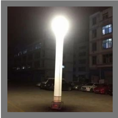
High Mast Emergency Light
