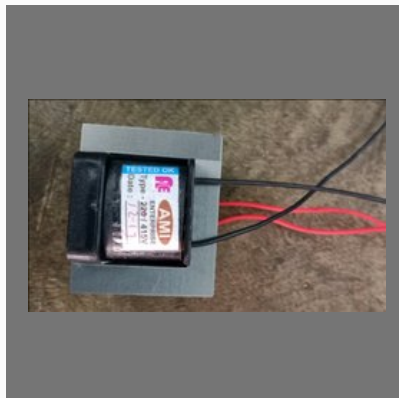
Double Phase Transformer
