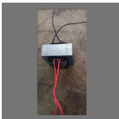
Single Phase Transformer
