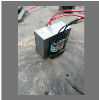
Single Phase Transformer
