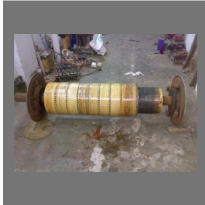
250kv Motor Repairing
