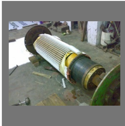
250 kw Motor Repairing
