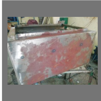
Panel Board Fabrication
