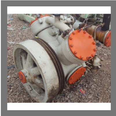
Kirloskar Ammonia Compressor
