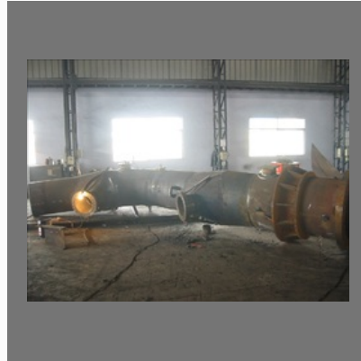
Distribution Pipe for Pelton Turbine
