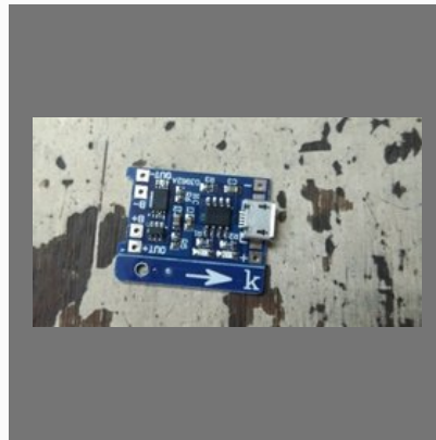
3.7 Volt Battery Charging Circuit
