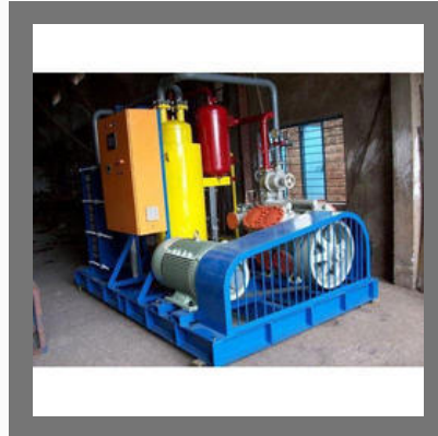
Expandable Ammonia Chilling Machine
