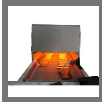
IR Drying oven for Adhesive Bonding
