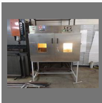
Infrared Oven for Softening COPE/HDPE Sheet for artificial Limbs
