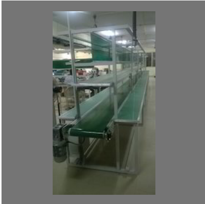
Conveyor With Working Desk
