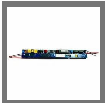
24 VAc/Dc to 32volt dc to80v dc 210 mA LED Driver
