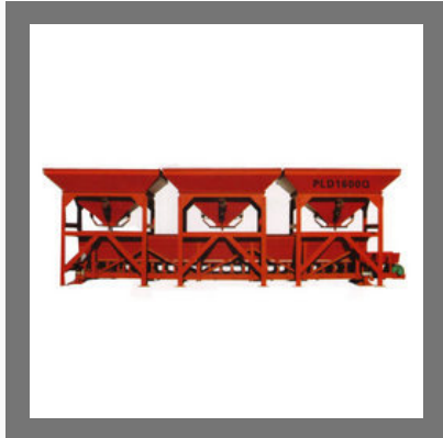
Concrete Batching Machine
