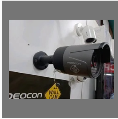
HD CCTV Camera
