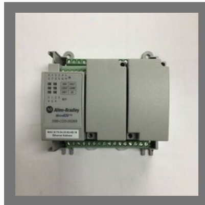
2080-LC20-20QWB Allen Bradley Micro820 PLC System
