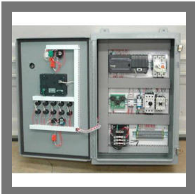
PLC Automation Control Panel
